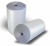
A continuous insulation solution that reduces radiant heat transfer for superior performance and a better alternative to foam board, especially in hot-humid climates. Perforated to allow vapor transmission and coated for long-term performance, the Flex Foam Low-e reinforced facing reduces up to 95% of radiant heat transfer to keep buildings cooler in the summer and warmer in the winter for greater comfort year-round.
