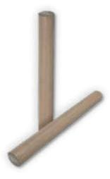
FSK Shield™ is a cost-effective radiant insulation solution with a single-sided Low-e foil facing reinforced with fiberglass scrim bonded to natural kraft paper. FSK can be used alone or in combination with other mass insulation and is commonly used as a Class A facing for unfaced batts or plenum ceiling applications. Adds up to R4.6 to exposed roof or ceiling systems. An easy, economical alternative to expensive foil-faced batts.
