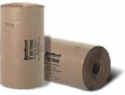
AA2 Vapor Shield™ is a radiant reflective insulation solution designed for masonry walls with wood furring or metal framing and can be used alone or in combination with other mass insulation. Gain cost-effective thermal performance by enhancing a minimum 3/4" enclosed cavity air space, providing R-value and potential to maximize livable area. 10-year transferable warranty. Perforated version recommended in hot-humid climates.
