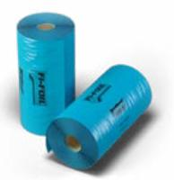
HY-Fi® is a multi-layered radiant reflective hybrid insulation solution for frame walls and can be combined with any mass insulation for improved thermal performance, requires a minimum 1-1/2" cavity air space to provide a minimum R7; commonly used as a wall or ceiling system with spray foam to minimize excess waste and gain flexibility for last-minute wiring changes without sacrificing performance. 10-year transferable warranty. Perforated version recommended in hot-humid climates.
